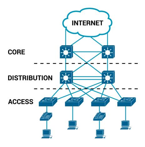
**Question 209.** Which of the following roles of campus switches provides an aggregation point for access switches?
