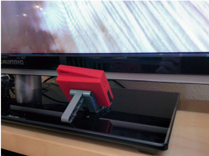
Fig. 4 Sensor on a small stand made of Lego by the participant to bring the sensor in optimal position in front of the tv set
