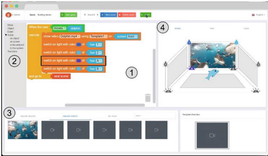
Fig. 11 MAT interface: (1) stage area, (2) actions and sensing components, (3) multimedia contents, (4) simulation area
