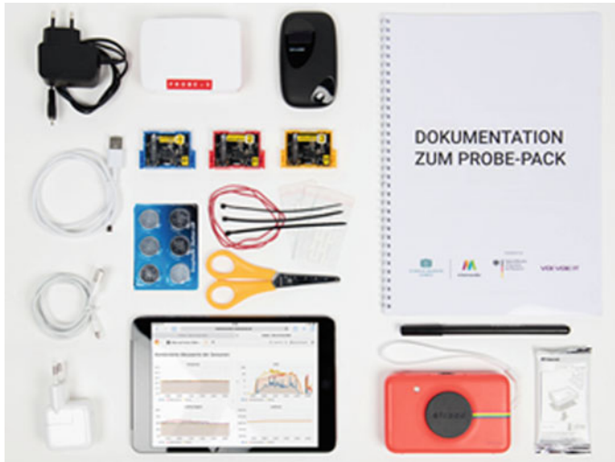
Fig. 1 Sensing Home Toolkit consisting of components for collection, processing, transmission and viewing of sensor data (3 SensorTags, Raspberry Pi, WiFi hotspot, tablet pc, etc.) with material for documentation and data work
