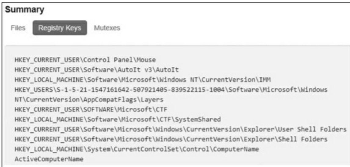
Figure 3-7: The Registry Keys tab of the Summary pane, showing which registry keys our malware sample modified
