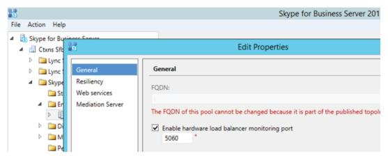
Once this change has been made, publish the topology to enable this port and create the custom NetScaler monitor. When creating this monitor, use SIP\_TCP as the protocol for the monitor as the NetScaler appliance supports Extended Content Verification using SIP\_TCP. For versions of NetScaler older than 10.5.e, you may use SIP\_UDP as the protocol. Optionally, you can create cus- tom monitors for the internal SIP virtual servers.
