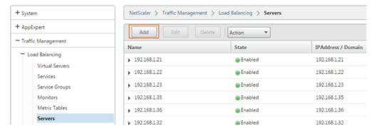
This will show the Create Server prompt, shown below. Provide a meaningful server name (or retain the IP address as shown below) and the IP Address of the server. All the servers that are being load balanced (Front End, Edge, Director or Database) should be added in this manner.
