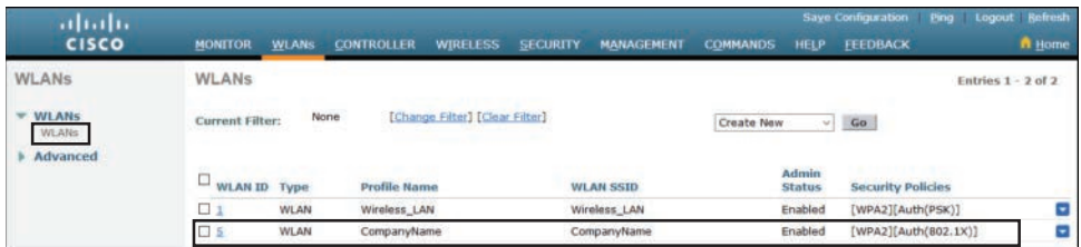
Figure 21-19 Verifying the New WLAN
