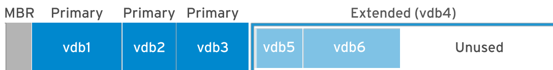
Figure 6.1: MBR Partitioning of the /dev/vdb storage device
